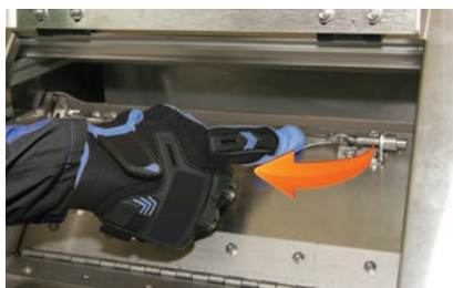
flip latch to open & close door
